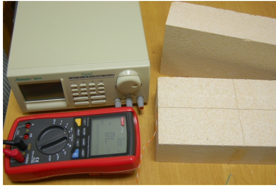
Figure 2: A simple equipment for the non-stationary hot-wire measurements (Brno University of Technology, Czech Republic).
